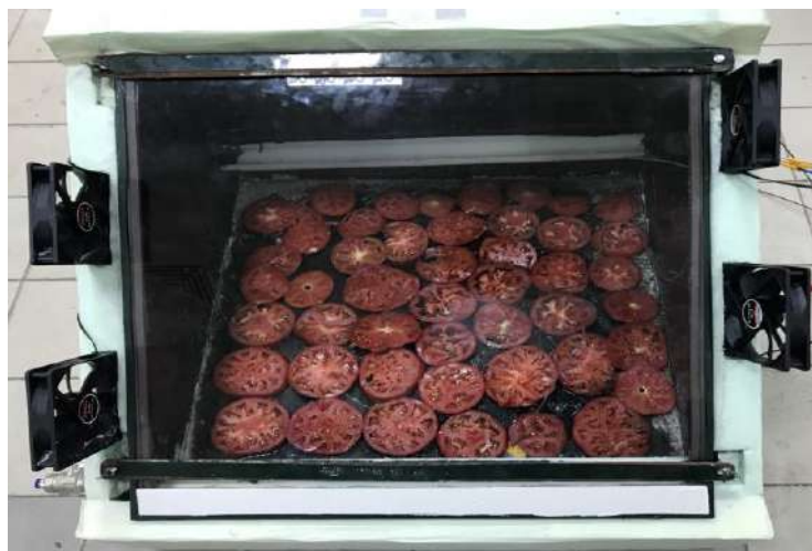
Figure 2. Filling the solar still with tomatoes
