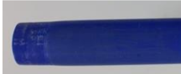
Figure 1: SDR 11 63 mm HDPE pipe used in tests
